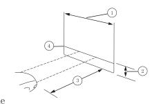
5. Locate the vertical adjuster on each headlamp. Using a Phillips #2 screwdriver, turn the adjuster either clockwise (to adjust down) or counterclockwise (to adjust up). The horizontal edge of the brighter light should touch the horizontal reference line.
